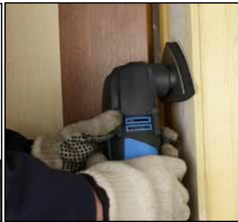
Demo of sanding using the sander head.
